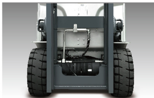
Front wheel dual drive motors offer stronger power
