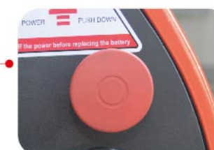
Emergency Power-off Switch
